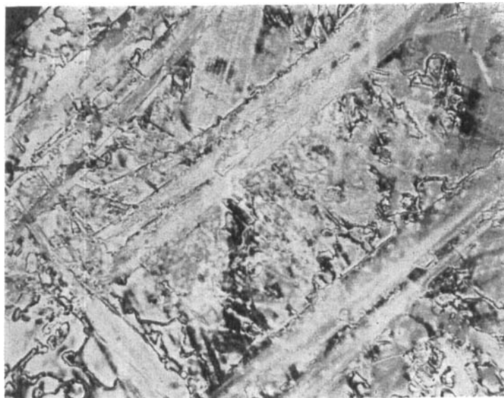
Figure 2. The smectic phase as it starts appearing in the nematic phase upon cooling. Temperature at the S-N point; magnification 100\times .
